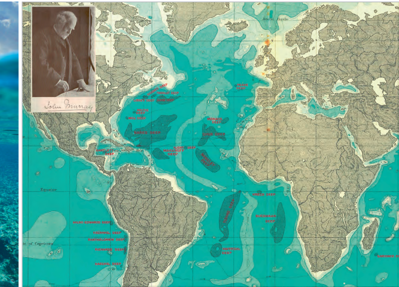
Fig 1: Sir John Murray and his 'bathymetrical chart' of the Atlantic, western Indian and eastern Pacific oceans published in 1912. Constructed from ~3,200 soundings made with pre-stressed hemp rope and lead weights on British and other survey ships. Abyssal plains ('deeps') correspond to depths >3,000 fathoms (5,486 m). Chart produced by John G. Bartholomew, cartographer to the King
