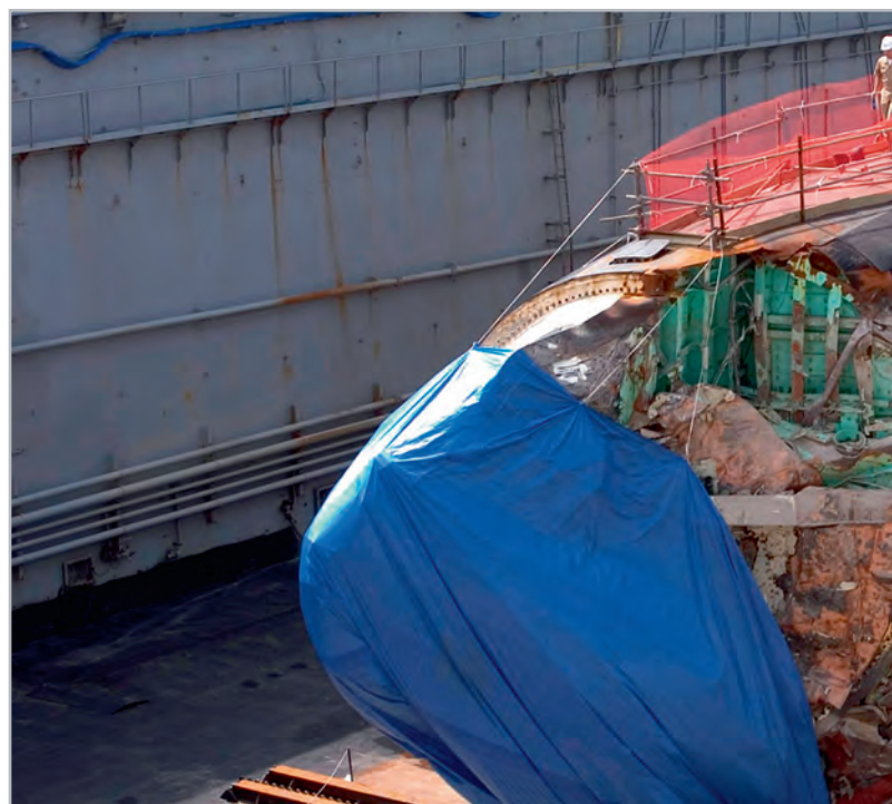
Fig. 9: USS San Francisco in Guam (Jan 2005). The submarine collided with an uncharted seamount while travelling at 33 knots between Guam and Brisbane. One sailor was killed, 115 were injured. (Credit: US Navy photo by Photographer O39, Mate 2nd Class Mark Allen Leonasio [Public domain])
